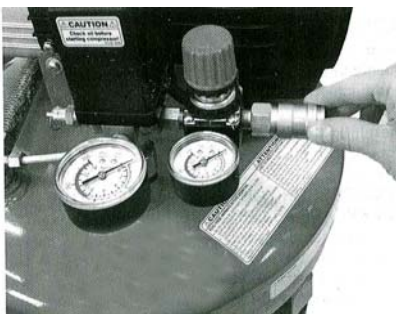
Figure 3 Installing the Air Chuck
