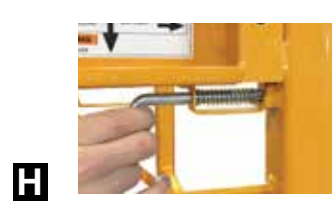
H Make sure that all four Lock Pins are secure and in LOCKED position.
