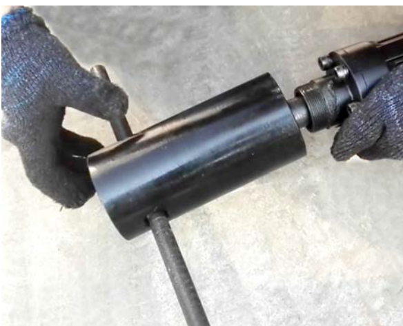
Fig. 5 ) To remove, insert Socket Pin then rotate Piling Socket Sleeve.
