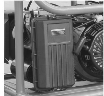
Figure 14 - Air Filter Casing.
