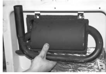
3. Remove Both Mufflers
