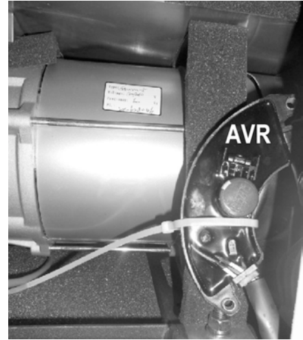
Figure B - Review the location of the AVR (Automatic Voltage Regulator. This item may eventually need to be replaced when they wear out.
