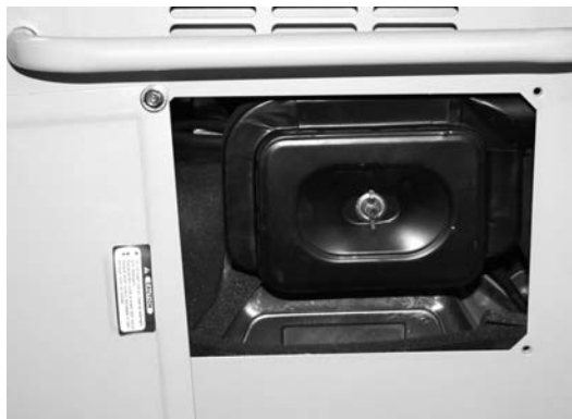
Figure 9 – Changing The Air Filter
