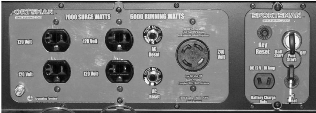
Figure 8 - Outlets Available on this Generator, from left to right, 120V AC, 240/120 AC and 12V DC.
