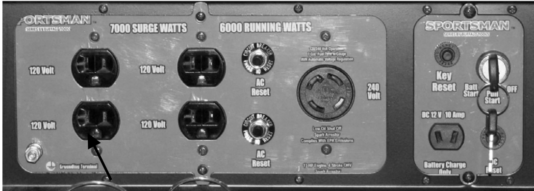
Figure 3 - Attaching the Grounding Wire to this Generator
