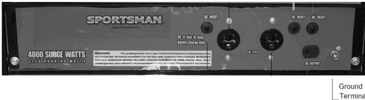
Figure 3 - Attaching the Grounding Wire to this Generator
