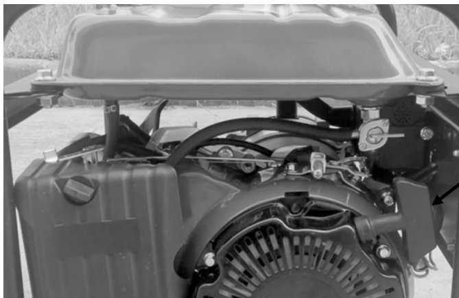
Figure 4 The Recoil Start is located on the left side of the generator.
