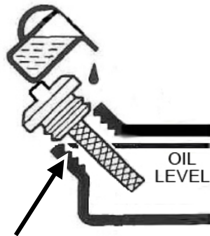
Figure 2 - Add Oil To TOP Of Threads
