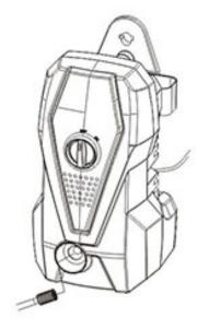
Attach Pressure Hose (#11) to the Pressure Washer.
