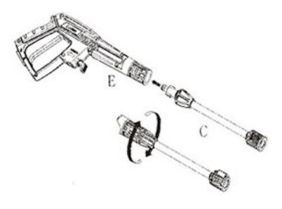
Attach the Gun Handle (E) to the Gun Lance (C).
