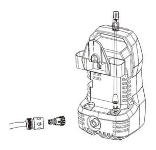
Attach your garden hose to the back of the Pressure Washer, using the quick connect.
