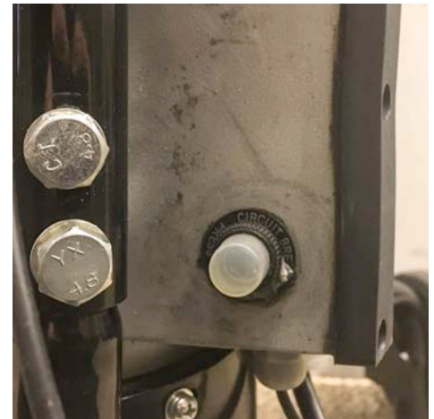
If you overload the motor, the unit will shut off automatically. Press the circuit RESET button to restart the motor.
