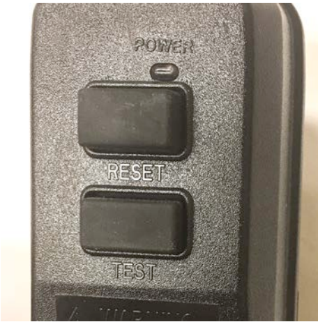
When you are ready to begin, insert the plug into an outlet. Then press the RESET button.
