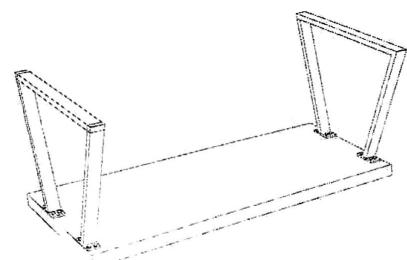
**3)** Position the remaining leg at opposite end. Secure each side with 4 hex bolts per leg.
