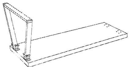
2) Place one set of legs at end of bench. Secure each side with 4 hex bolts per leg.
