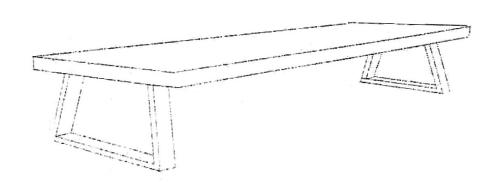
**4)** Securely tighten all hex bolts. Rotate bench.
