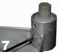
Each corner support requires two Hex screws. Wait until the table is completely assembled before securely tightening each Hex screw.
