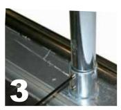
Using the Hex wrench, loosely tighten the Hex screws (with the HEX side visible) into the corner support.
