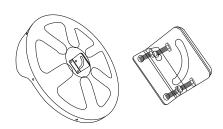
4. Adjust the left L part and right L part on the back of convex mirror, then add 4 pieces M6\*16 screws on the L parts and convex mirror.
