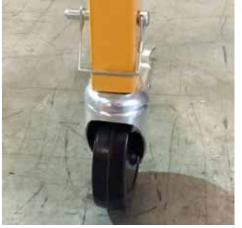
Use the Connector Pins (BB) to attach the Casters to Outrigger.
