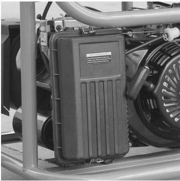
Figure 14 - Air Filter Casing.
