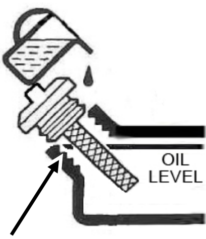
Figure 2 - Add Oil To TOP Of Threads
