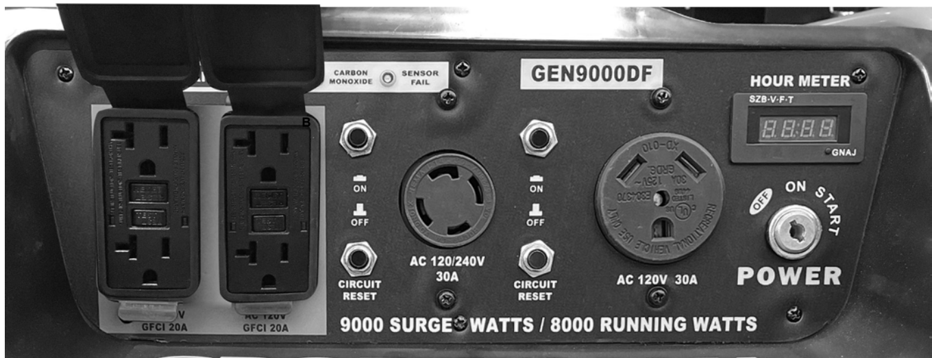
Figure 8 - Outlets available on this generator, from left to right: 4 each 120V GFCI AC , 120/240V AC, 120V AC RV.
