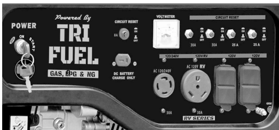
Figure 8 - Outlets available on this generator, from left to right: 12V DC, 120/240V AC, 120V AC RV, and 4 each 120V AC GFCI.
