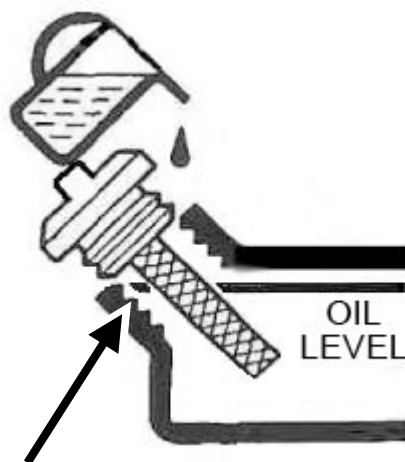
Figure 2 - Add Oil To TOP Of Threads
