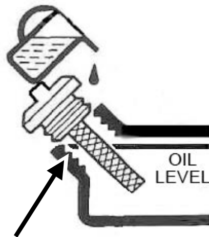
Figure 2 - Add Oil To TOP Of Threads
