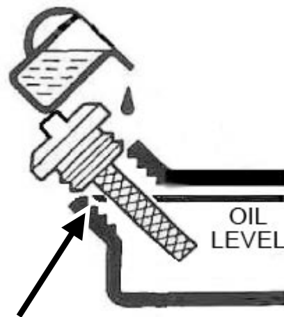
Figure 2 - Add Oil To TOP Of Threads
