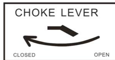
Figure 5 - Choke Lever in the “closed” position. (Refer to the Generator Components chart to find the location of the Choke Lever.)
