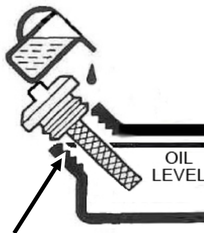
Figure 2 - Add Oil To TOP Of Threads
