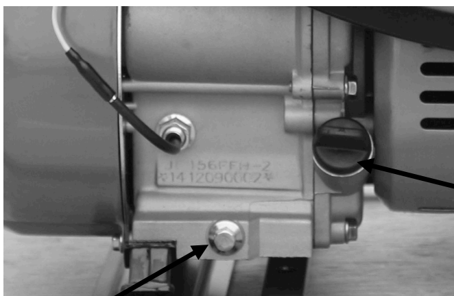
Figure 8A – Use 12mm hex wrench to REMOVE bolt and drain oil
