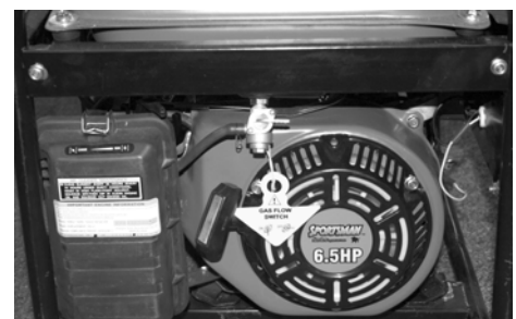
Figure 4 The Recoil Start is located on the left side of the generator.
