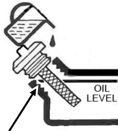
Figure 2 - Add Oil To TOP Of Threads
