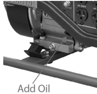
Figure 11 - Checking the Oil
