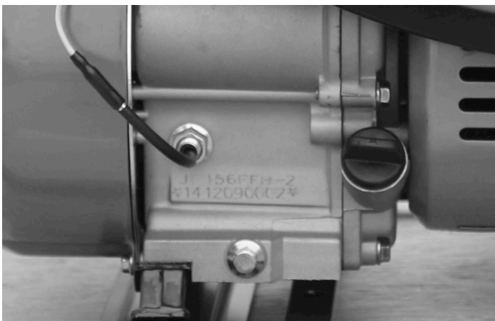
Figure 1 – Unscrew the Dipstick Cap
