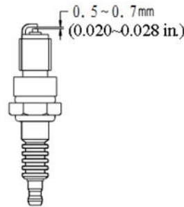
Figure 9 Measuring the spark plug gap
