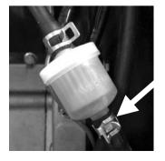
Remove fuel line from filter. Fuel will drain from both bowl and fuel line.
