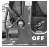
Rotate gas valve to "OFF" position.
