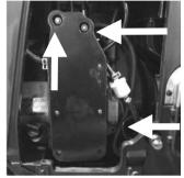
Remove three screws from engine air box
