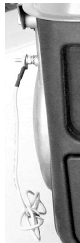
Figure 3 The Grounding Terminal is located on the side of the generator.
