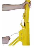
3. Feed the free end of the cable under and around the winch hub, then through the hole into the winch drum.
