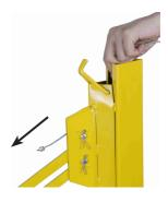
2. Pull the cable through the sheave pocket, and slide the new telescoping sections down into the frame.
