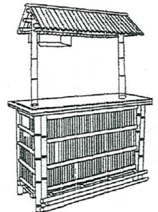
Figure 6 Add the Hanging Rack (#13), then tighten all bolts and screws to secure the Bamboo Bar.
